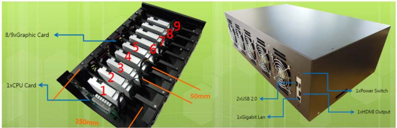
Figure A. A mining rig comprised of NVIDIA GPUs Source: NVIDIA Corp.
