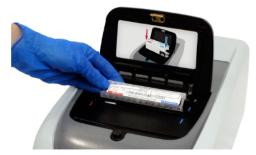
Position the pouch with the black array on the right side and the film portion of the pouch entering the instrument first. The pouch will lock into place when it is properly inserted.
