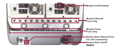
33. The Ethernet interface to which a programmable processor of the FilmArray Torch Module connects is a communication assembly.
