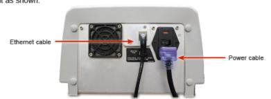
Connect the instrument Ethernet cable and instrument power cord to the back of the instrument as shown.
