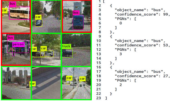
Figure 7: Left: A challenge images with detected bounding boxes. Right: Filtered JSON output returned by the bounding box to grid mapping algorithm. The target object is a bus.
