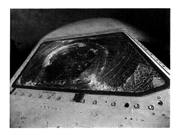
Figure 7-12: Photograph of windshield damage
