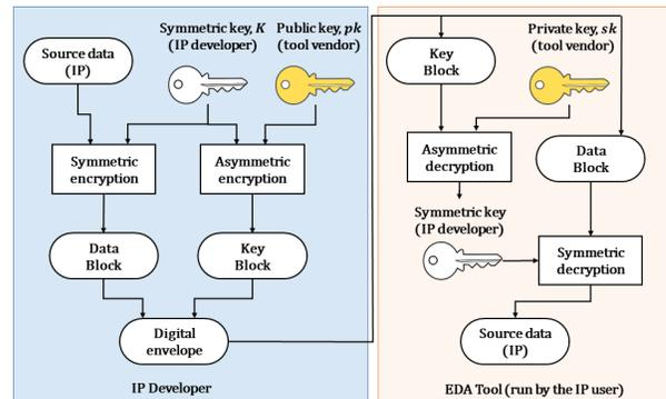
Figure 3: Work flow of the P1735 standard.
