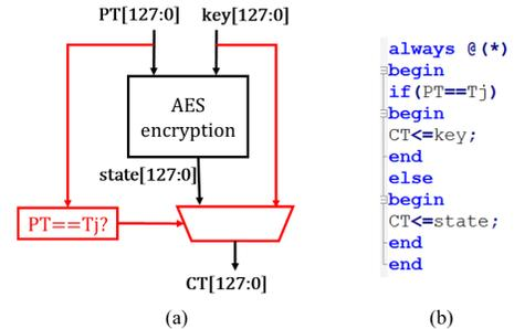
**Figure 7:** (a) Schematic of a Trojan which leaks the on-chip private key used by the AES IP. (b) The Verilog code which implements this Trojan.
