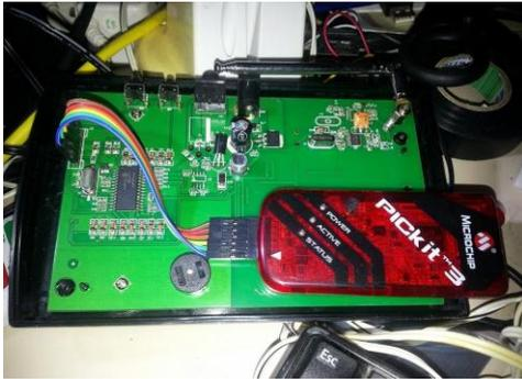
It is hard to stop attackers with physical access. The marking on the IC could be removed that would make it more difficult for an attacker. It should be assumed that physical tampering and reversing may be attempted but it is very hard to stop a well resourced attacker.
