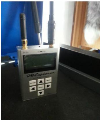
programs can both show signal strength and demodulate the signal using AM or FM.
