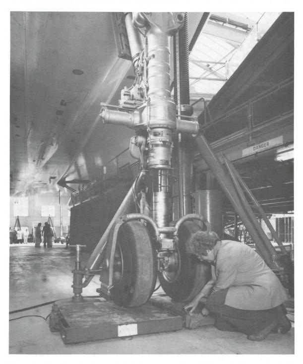
Concorde is shown being weighed by means of weighing-platforms beneath each landing wheel. The weighing-platforms have been calibrated at NPL. All aircraft must be weighed to conform to an Air Navigation Order.
