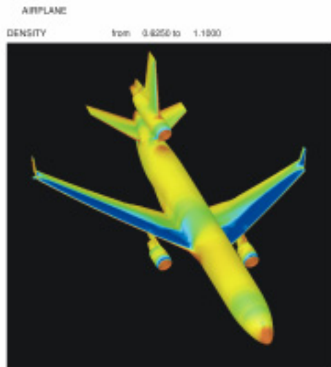
Figure 7. Density contours for the MD-11.
